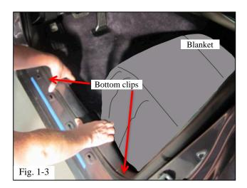
(e) Remove the front driver's inner door sill trim (Fig. 1-3).
