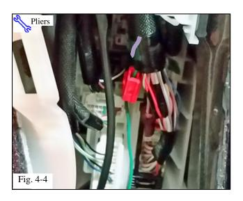
(h) Apply a wire tap to the violet wire and connect the green wire from the electronics module to the wire tap (Fig. 4-4).
