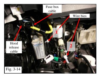
(r) Continue running the wire along the foot lamp harness and secure it with two (2) wire ties as shown. Make sure to route above the hood release and fuse box cables (Fig. 3-14).
