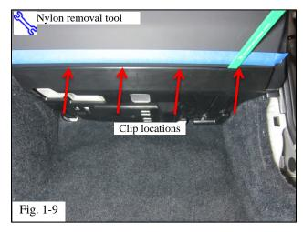
(1) Place masking tape, unless protected, on the bottom edge of the passenger's side knee panel. Use a nylon removal tool to release the 4 clips as shown on the lower trim panel (Fig. 1-9).
