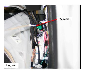
(l) Run a long (blue) wire from the electronics module up along the vehicle wire harness and secure it with one (1) wire tie (Fig. 4-7).
