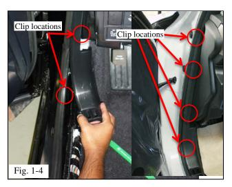
(f) Remove the kick panel trim piece from the vehicle by pulling rearward to disengage the four (4) clips while holding the weather strip at the clip locations (Fig. 1-4).
