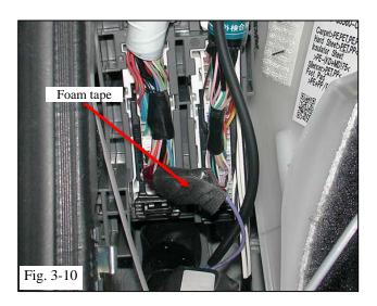
(n) Reattach the black lock mechanism and reconnect the connector to the connector block (Fig. 3-10).
