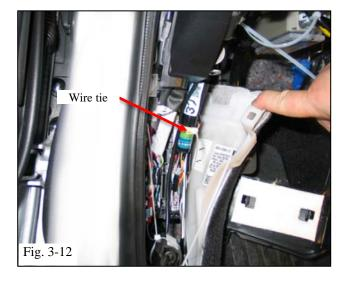
(p) Run a long (blue) wire from the electronics module up along the vehicle wire harness and secure it with one (1) wire tie (Fig. 3-12).
