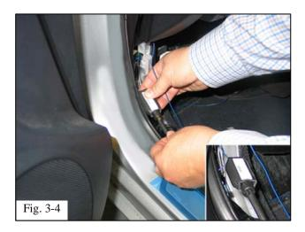
(f) Insert the optical wire harness from the door sill into the opening on the electronics module until it clicks into place (Fig. 3-4). Lightly tug on the wire harness to insure it is locked in.
