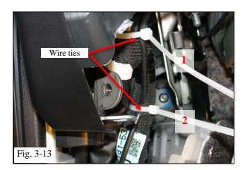
(q) Continue running the wire up and secure it with two (2) more wire ties (Fig. 3-13).
