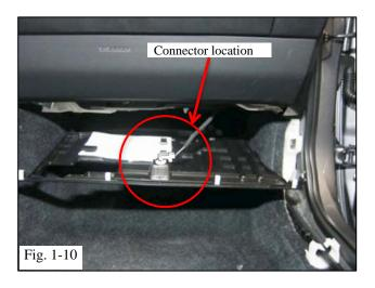
(m)Lower the panel to expose the foot light connector. Disengage the connector and remove the panel. Remove the masking tape.Make sure no tape residue is remaining (Fig. 1-10).
