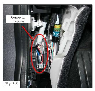
(g) Locate the 67 pin connector on the driver's side kick panel connector block (Fig. 3-5).
