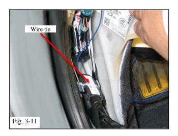
(o) Secure the electronics module and harness to the existing vehicle harness with one (1) wire tie (Fig. 3-11).
