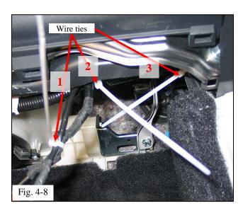
(m)Continue running the wire up and along the foot lamp harness and secure it with three (3) wire ties (Fig. 4-8).
